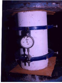
Figure 1: Test set up for cylinder
