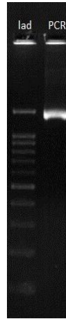
figure 1: A single discrete PCR amplicon band of 1500 bp was observed when resolved on Agarose gel.
