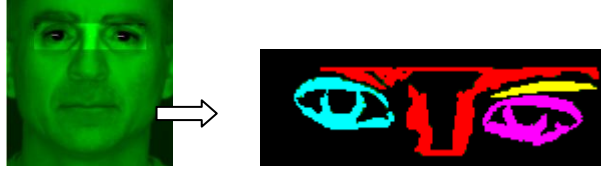
Fig:8 Finding the Eye Parameters. a) Normalise locally, b) Use edge detection and blob analysis
