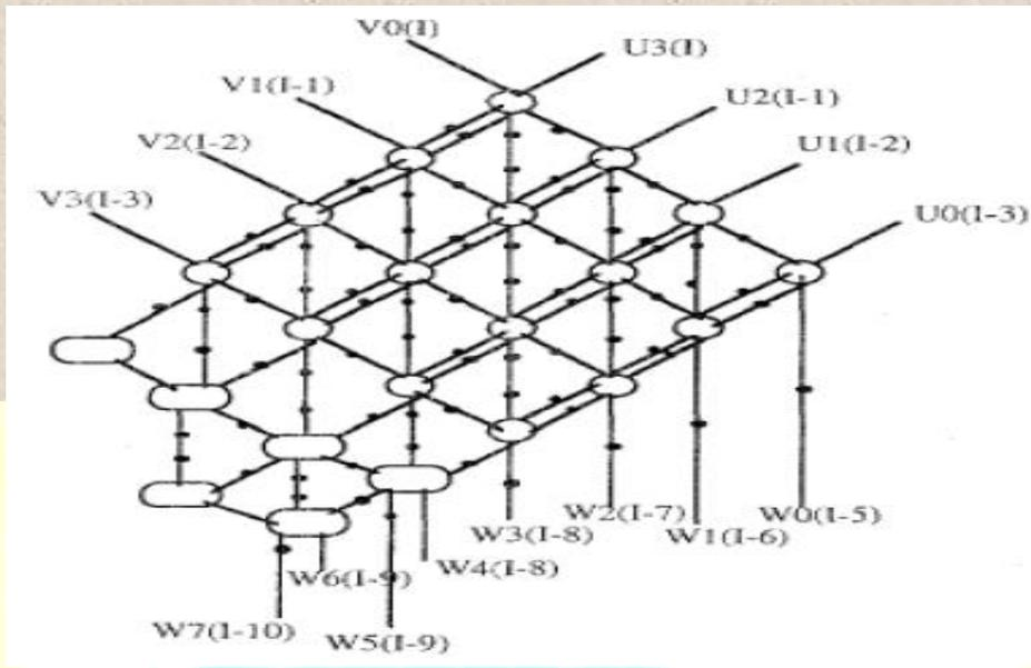
Fig 2: Radix 2n architecture
