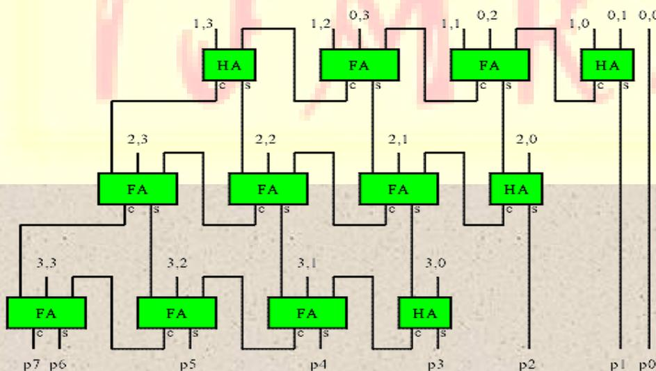
Fig1: 4x4 array multiplier
