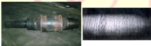
Fig.5 Damaged Casting Roller with Thermal Cracks
