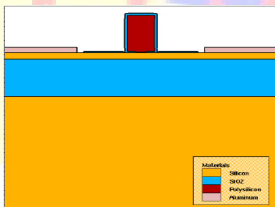
Fig. 3 Final SOI structure obtained by process simulation in Athena Simulator
