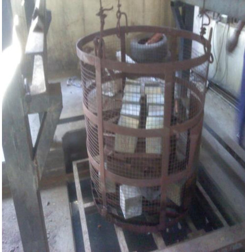
Photo 5. Placing of Specimens in Furnace
