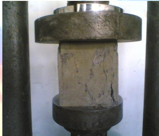
Photo 8. Compression test on concrete cube
