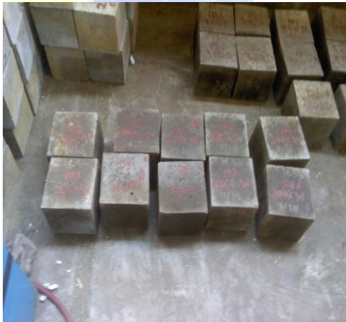
Photo 7. Specimens at dry cooling condition after elevated temperature
