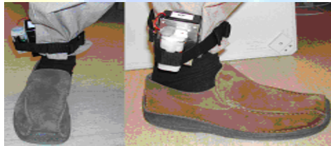
Figure 5: The Gait Collector attached to a person’s leg in its ideal position just above the right foot’s ankle.
