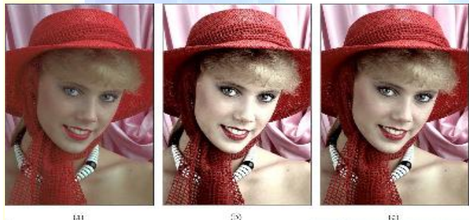
Fig.14. Results for image Face . (a) Original image, (b) enhanced image obtained using HE, (c) enhanced image obtained using WTHER,
