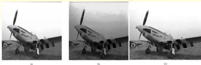
Fig.7. Results for image Plane . (a) Original image, (b) enhanced image obtained using HE, (c) enhanced image obtained using WTHE
