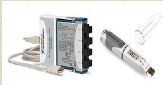
Figure 2. Data loggers can be both PC-based or stand-alone devices.
