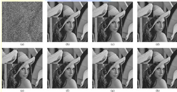
Fig. 4. Restoration results of different filters. (a) Corrupted Lena image with 80% salt-and-pepper noise (6.42 dB). (b) Original image. (c) CM filter (28.66 dB). (d) MMEM filter (27.66 dB). (e) AM filter (24.89 dB). (f) BDND filter (27.67 dB). (g) FM filter (23.08 dB). (h) AM-EPR filter (27.23 dB).
