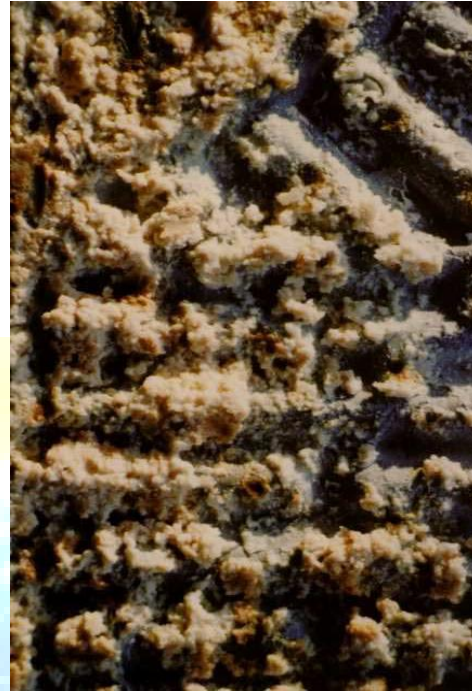
Figure.1 - Crystalline (Milkstone) Fouling on a Plate and Frame Exchanger Plate from the Dairy Industry
