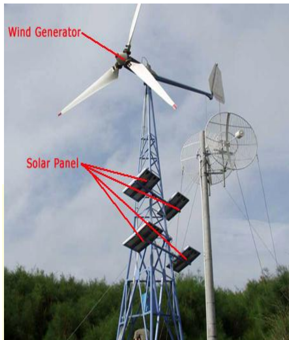
Fig.6 Hybrid solar and wind power system
