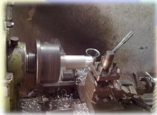
*Fig 4.14: Turning Operation*
