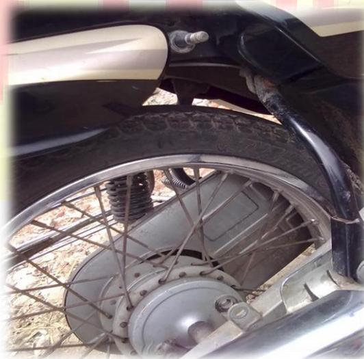
*Fig 4.22: Bike with Shock Absorber removed*
