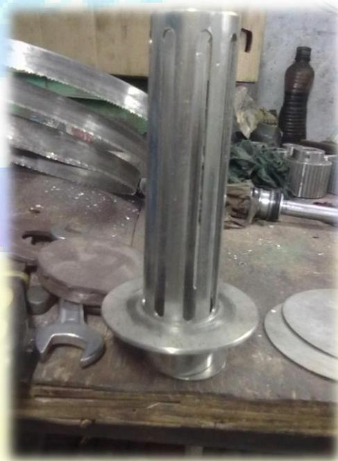
*Fig 4.16: Finished Coil Support Tube*
