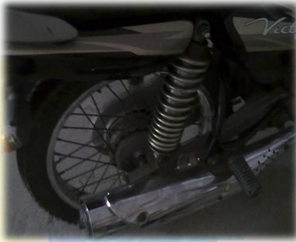
*Fig 4.23: Regenerative Shock Absorber attached to the vehicle*
