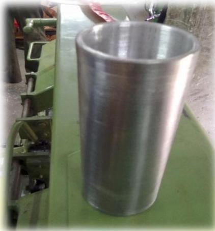
*Fig 4.18: Aluminum Dust Cover (After Turning)*
