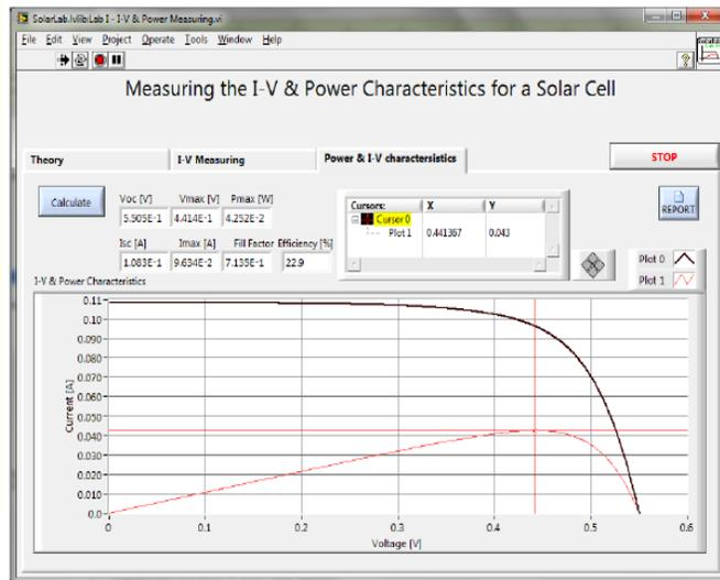
Fig.22 I-V and Power-Measuring Interfaces
