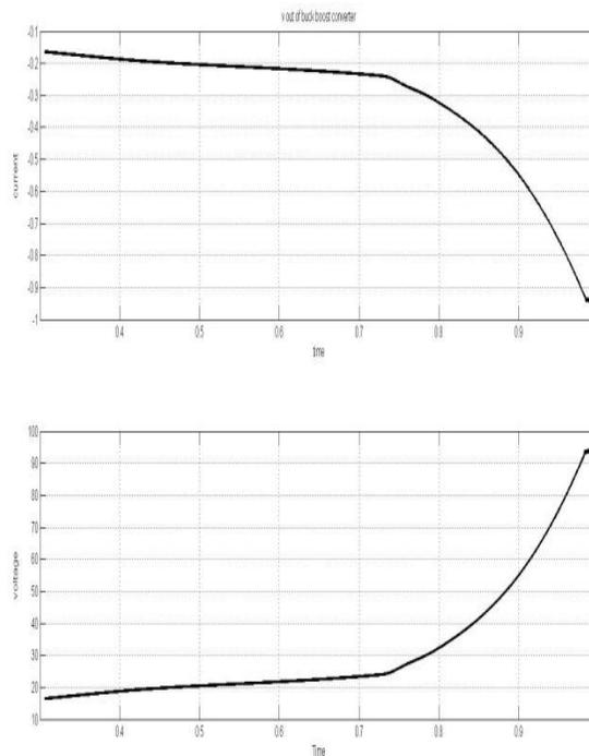
Fig.14: Output voltage across the buck boost converter
