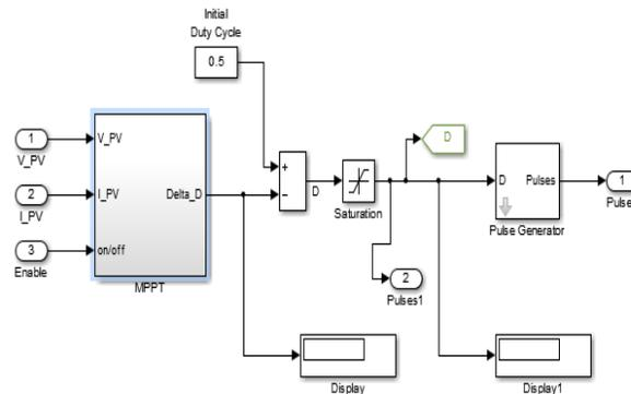
Fig.10: Pulse generator using MPPT block Modeling and for buck boost converter
