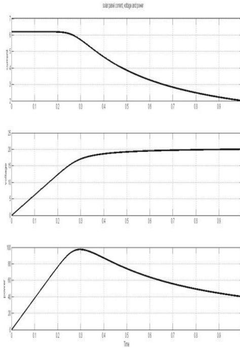
Fig .12: output of solar panel current, voltage and power
