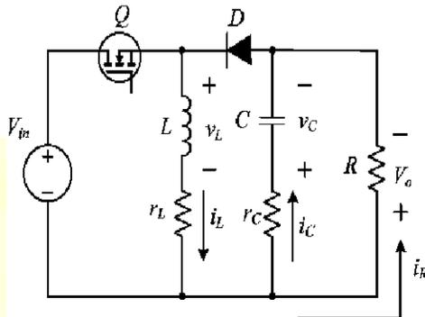
Fig.11: DC-DC Buck Boost converter circuit diagram
