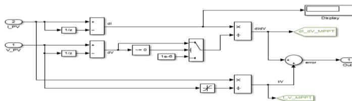
Fig 8: MATLAB-Simulink model implementing incremental conductance method
