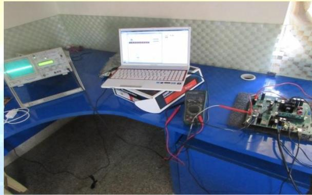
Fig.15: Experimental setup of TMS320 solar explorer kit
