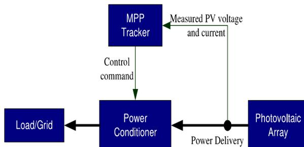
Fig.6 Block diagram of Maximum power tracking system
