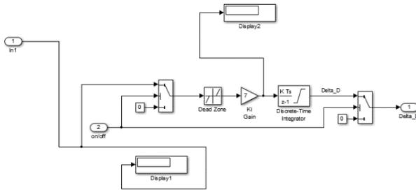
Fig.9: MATLAB-Simulink model of pi controller for MPPT model
