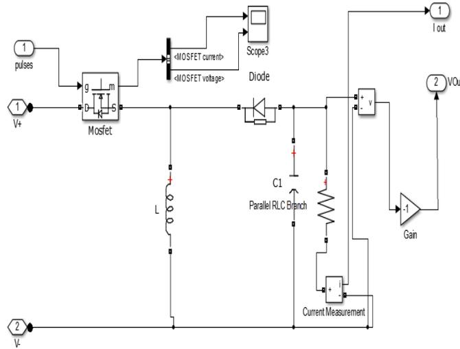
Fig.4.14: Simulink model of buck boost converter
