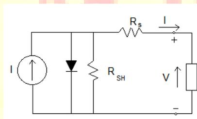
Fig.4: Single diode model of a PV cell
