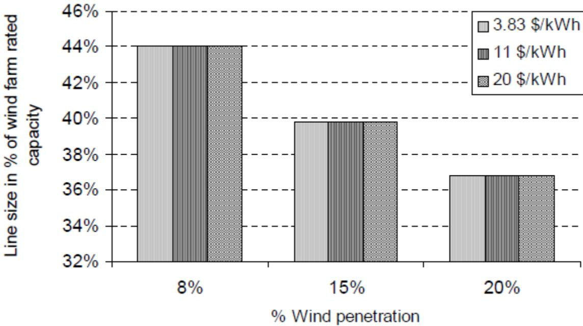
Fig. 5.5 Cost effective line sizing with varying IEAR
