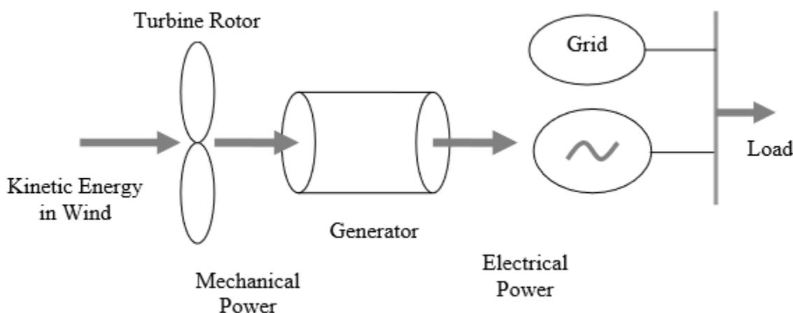
Fig. 3.2 General principle of WECS
