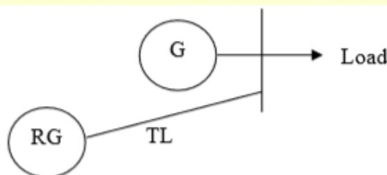
Fig. 2.4: HL-I system model incorporating transmission line
