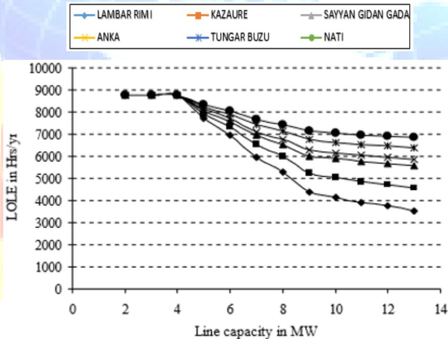
Fig. 4.8: Variation in LOLE with line capacity for 13 MW peak load
