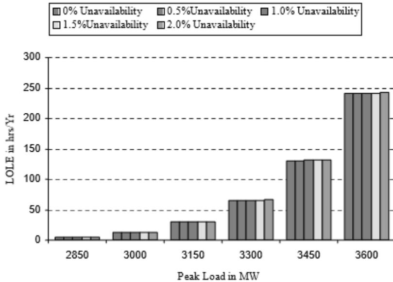
**Fig. 4.13:** System risk versus peak load for 250 MW line capacity and varying transmission line availability
