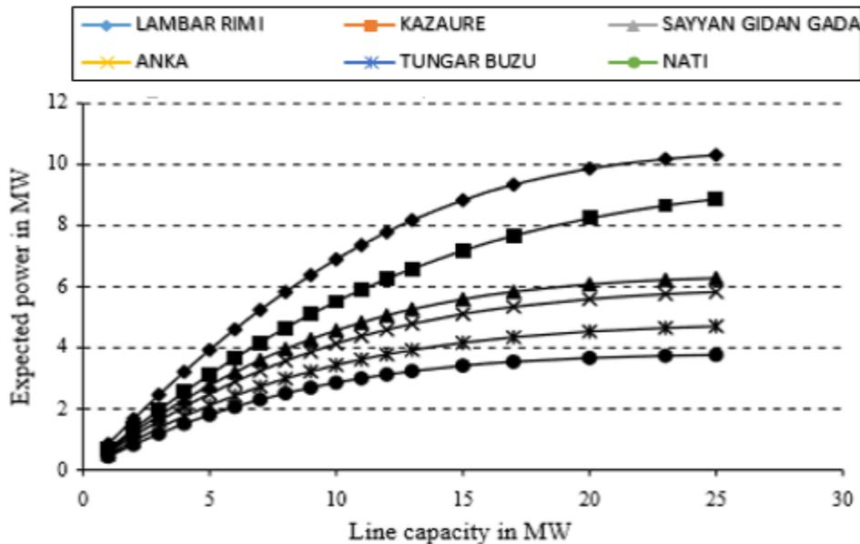
Fig. 4.9: Variation in EPO with line capacity for different wind regime
