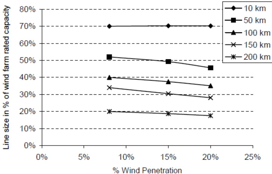
**Fig.5.6** Cost effective line size for varying line length
