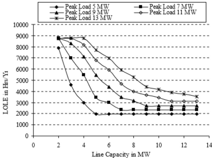
Fig. 4.4: Variation in system LOLE with line capacity
