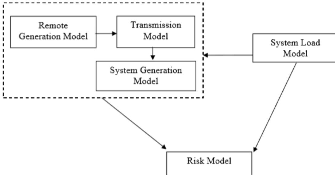
**Fig. 2.5:** Evaluation model incorporating transmission system in HL-I
