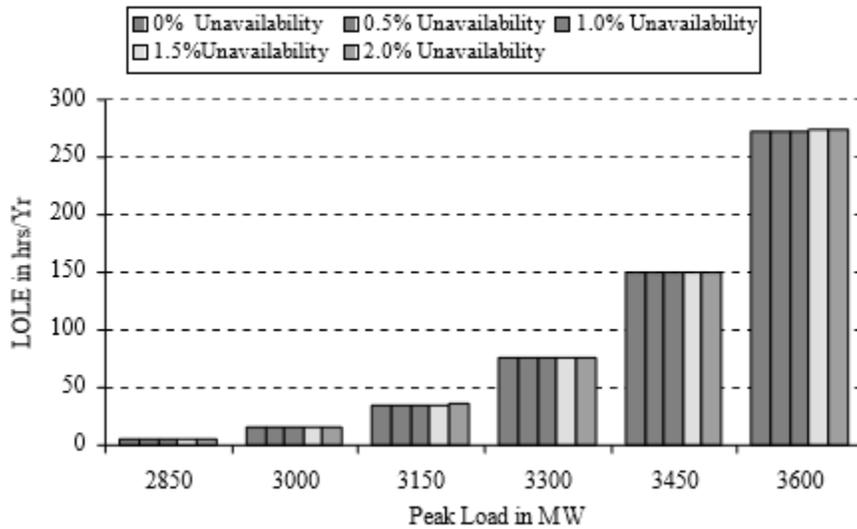
**Fig. 4.12:** System risk versus peak load for 50 MW line capacity and varying transmission line availability
