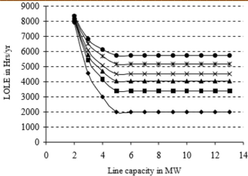
Fig. 4.7: Variation in LOLE with line capacity for 5 MW peak load
