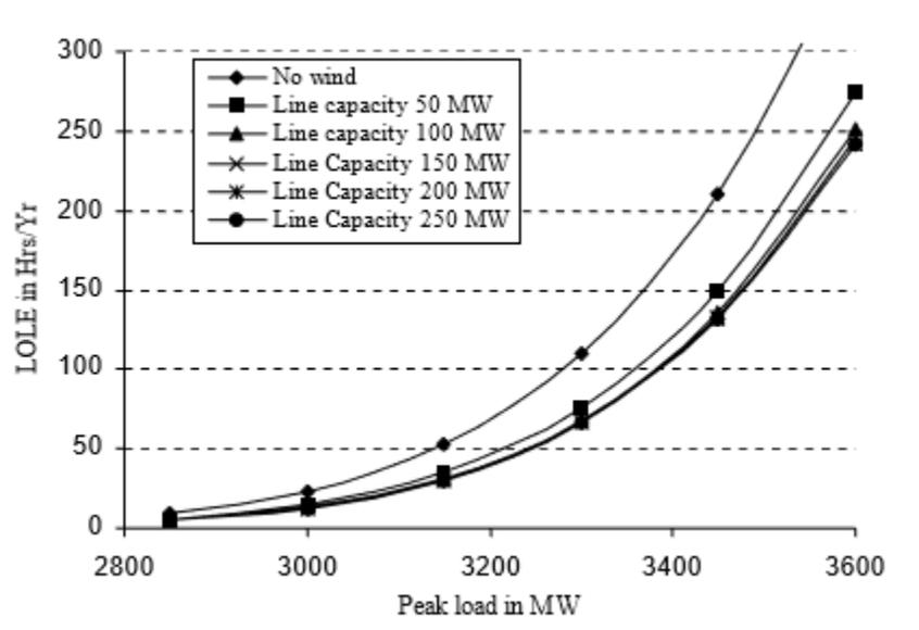
Fig. 4.11: System risk versus peak load with varying line capacity
