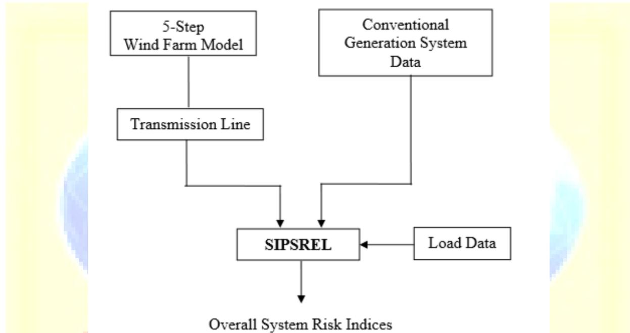
**Fig. 3.7:** Application of SIPSREL in adequacy evaluation
