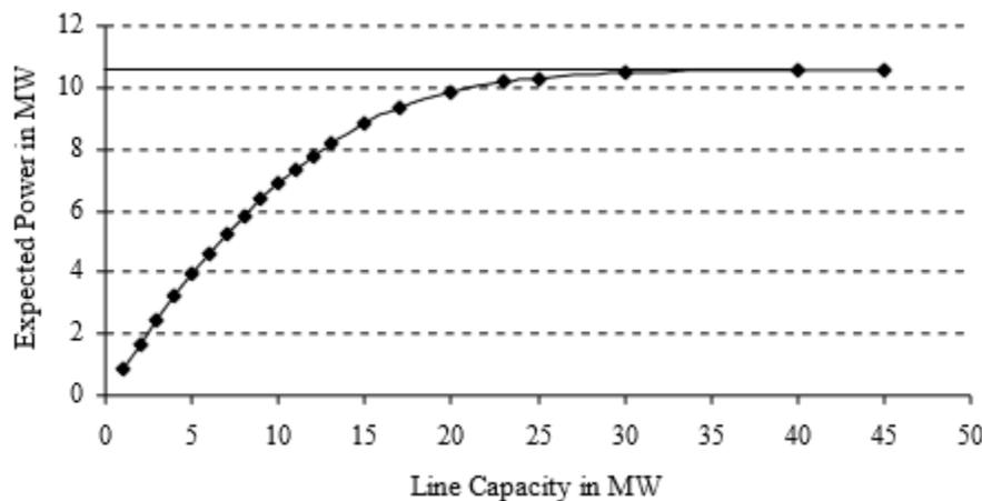
**Fig. 4.5:** Variation in system EPO with line capacity
