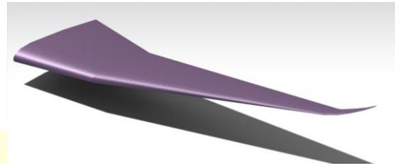
**Fig. 7: Wing with Racked wingtip**
