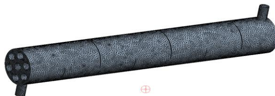
Plate II: Meshing of Heat Exchanger
