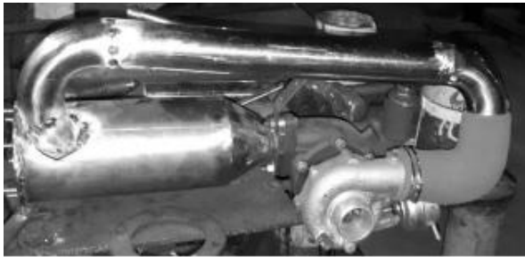
Figure 3: Mounting of combustor on The Turbocharger
