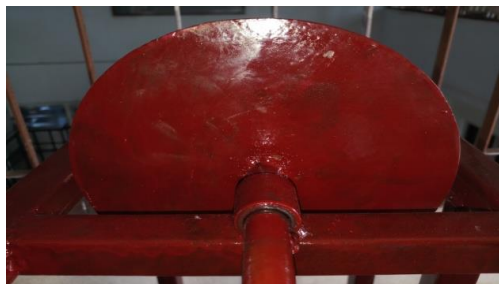
Fig 6. shaft with eccentric plate
