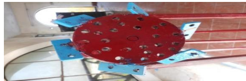
Fig3. Hub with mid steel plates on it
