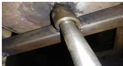
Fig4. Plain bearing with shaft in it
