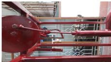
Fig8. Eccentric plate with piston pump
