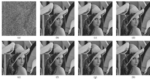
Fig.3 Restoration results of different filters. (a) Corrupted Lena image with 80% salt-and-pepper noise (6.42 dB). (b) Original image. (c) CM filters (28.66 dB). (d) MMEM filter (27.66 dB). (e) AM filter (24.89 dB). (f) BDND filter (27.67 dB). (g) FM filter (23.08 dB). (h) AM-EPR filter (27.23 dB)
