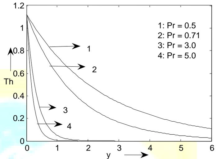
Fig.10: Temperature profile for different values of  $Pr$
