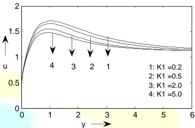
Fig. 6: Velocity Profile for Different values of K1
