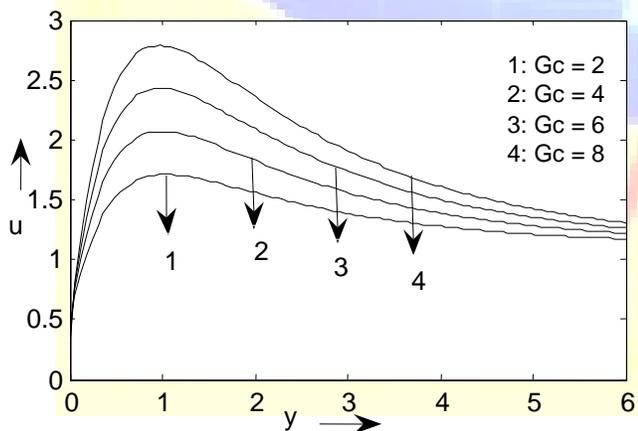
Fig. 7: Velocity profile for different values of Gc
