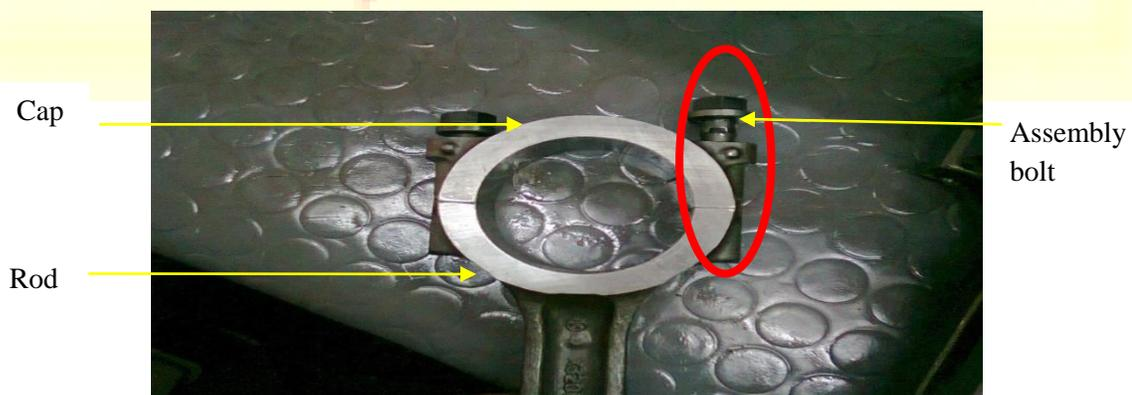
Photograph of Cap & Rod assembly bolt tight problem
