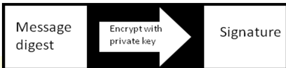
Figure 6 Encryption Of Message Digest Into Signature
