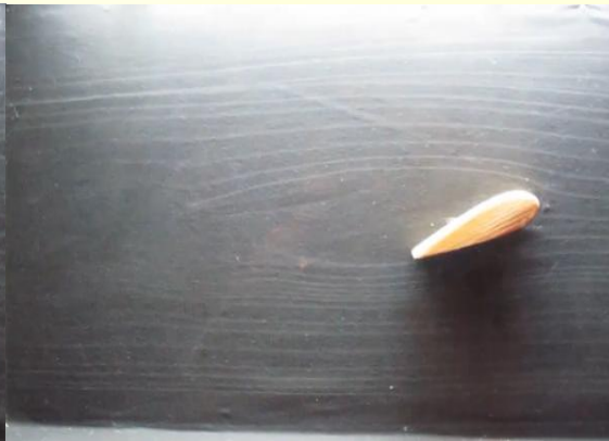
Fig 5.3(b): Flow past an aerofoil with non-Zero angle of attack
