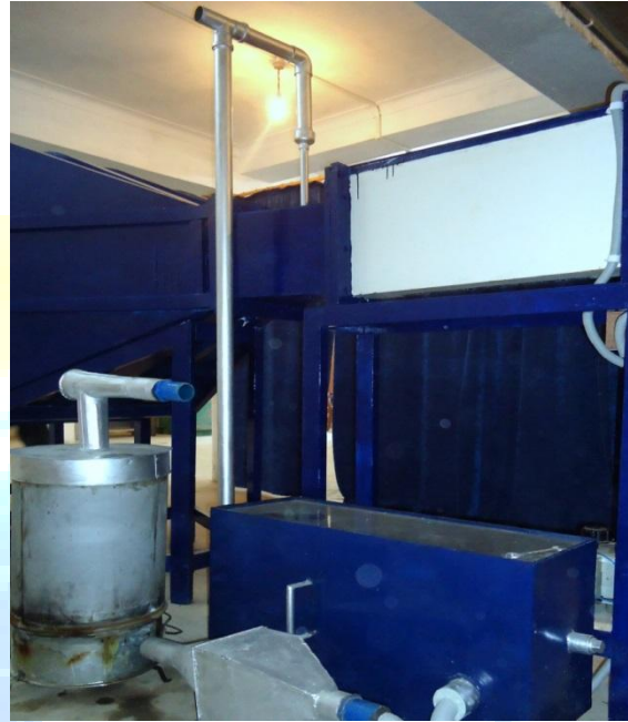
Fig 2.2: Smoke generator and smoke circuit
