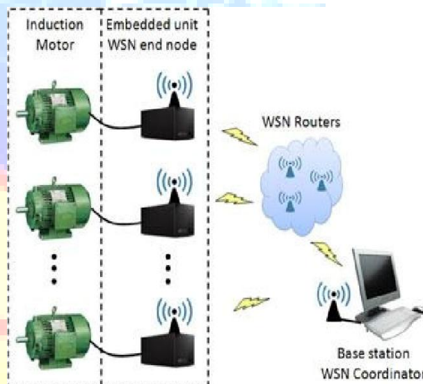
Figure. 2 Embedded systems integrated into WSN
